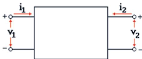
$$\begin{cases} i_1(t) = \gamma \cdot v_2(t) \\ i_2(t) = -\gamma \cdot v_1(t) \end{cases}$$
